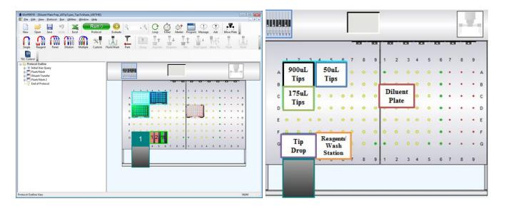
10. You can check or uncheck which portions of the protocol to run. Browse to choose the appropriate worklist file which will be created when you calculate the amounts of diluent to deliver.
