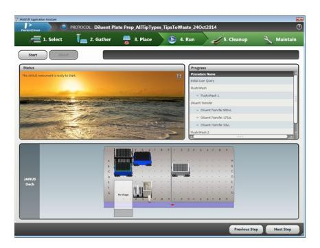
12. Ensure that all tip boxes are filled, then press ok to run the protocol.
